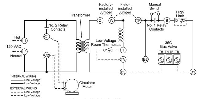
Figure 4. 24 Volt AC Gas Valve
